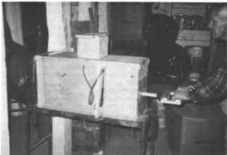
Fig. 1. Plywood Double-Action Piston Pump, with manometer attached for tests.
