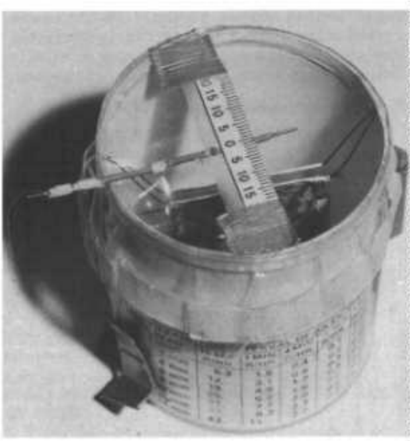
Fig. 10.1. A homemade KFM, an accurate dose rate meter for measuring dose rates from 30 mR/hr (0.03 R/hr) up to 43 R/hr.
